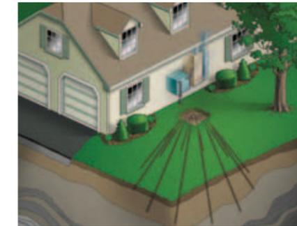
Ground source heat pumps work by exchanging heat energy with the earth at depths of one to 100 metres, using a loop field which can be installed horizontally or vertically. Images courtesy Geo Climate Systems and WaterFurnace (left) and Dr Donald Payne (right)
