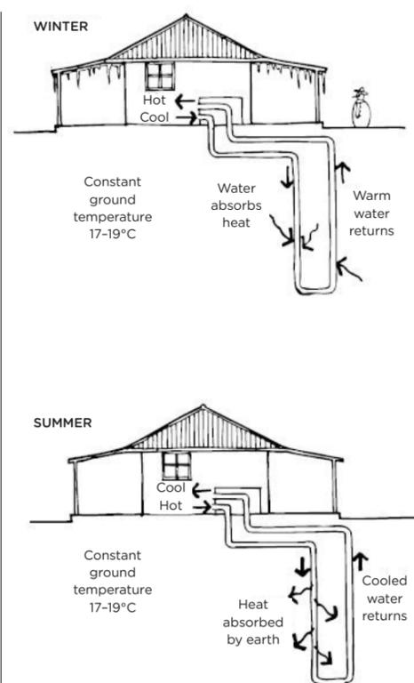
A ground source heat pump uses the relatively constant ground temperature to warm the system's circulating liquid in winter, and cool it in summer. It's then used for functions like heating and cooling the home and providing hot water. Image courtesy Your Home Technical Manual
