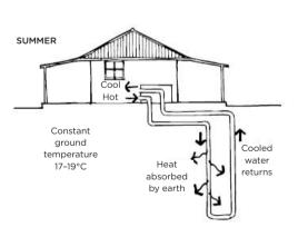
A ground source heat pump uses the relatively constant ground perature to warm the stem's circulating liquid winter, and cool it in summer. It's then used for functions like heating and cooling the home and providing hot water. age courtesy Your Home Technical Manua
