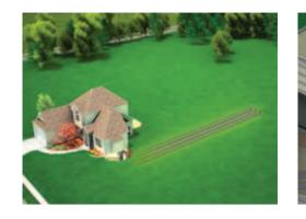
degrees as its starting point and only has to work to heat the air within the house by two to four degrees. A conventional electric heat pump (such as reverse cycle air-conditioning) in the same house, on the other hand, would take the outside air temperature of five degrees Celsius as its starting point and would need to work harder, using more electricity, to heat the air within the house by 14 degrees to have the same effect.
