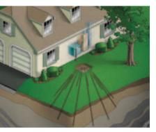
Ground source heat pumps work by exchanging heat energy with the earth at depths of one to 100 metre using a loop field which car be installed horizontally or ertically. Images courtes Geo Climate Systems and terFurnace (left) and Dr Donald Payne (right)
